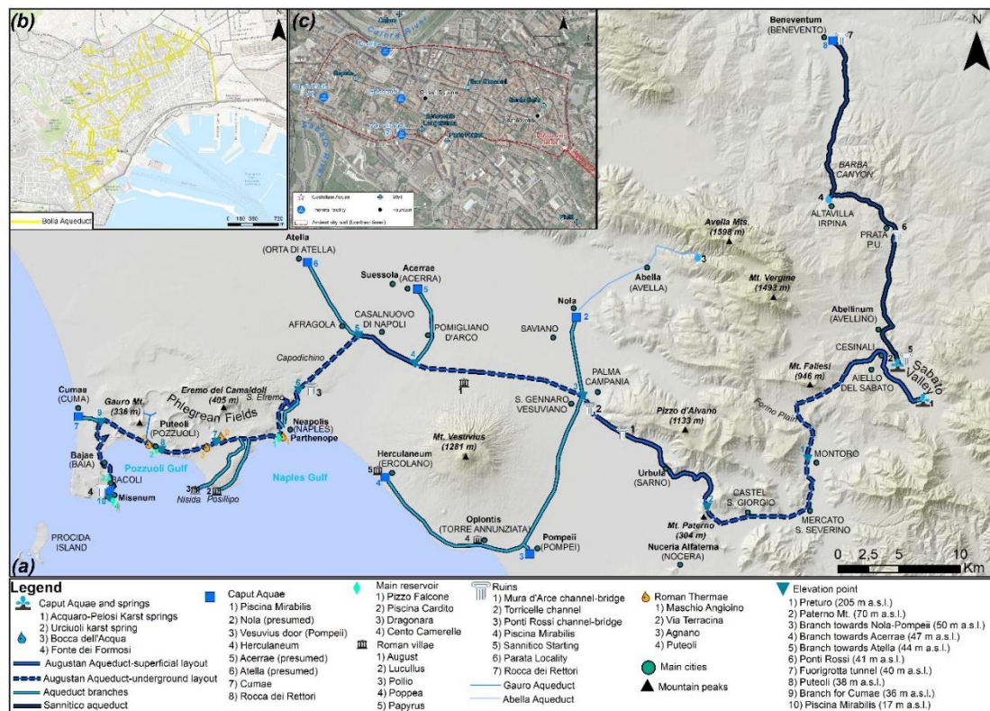
Layout of Roman Aqueducts tapped Serino springs (from Esposito et al., 2025-modified)
