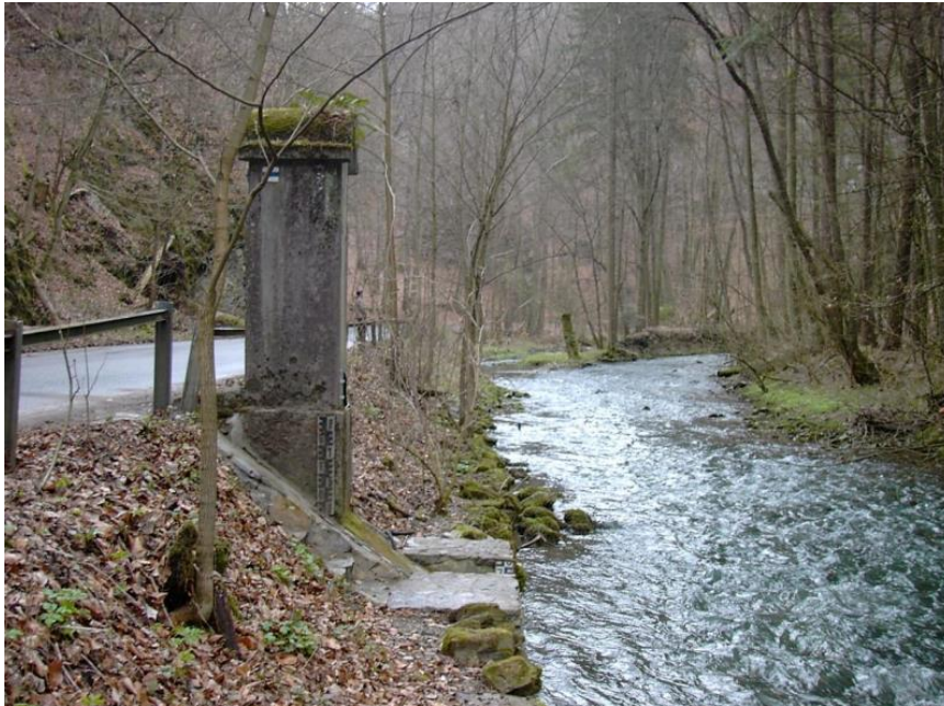
Gauging station on the Punkva River in the Moravian Karst operating since 1923. In the background, the confluence of the Punkva River outflow from the drainage tunnel (photo by Peter Malik)
