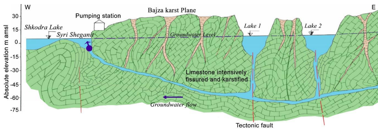
Cross-section A-A, through Blue Eye Spring (after Eftimi R. 2008)
