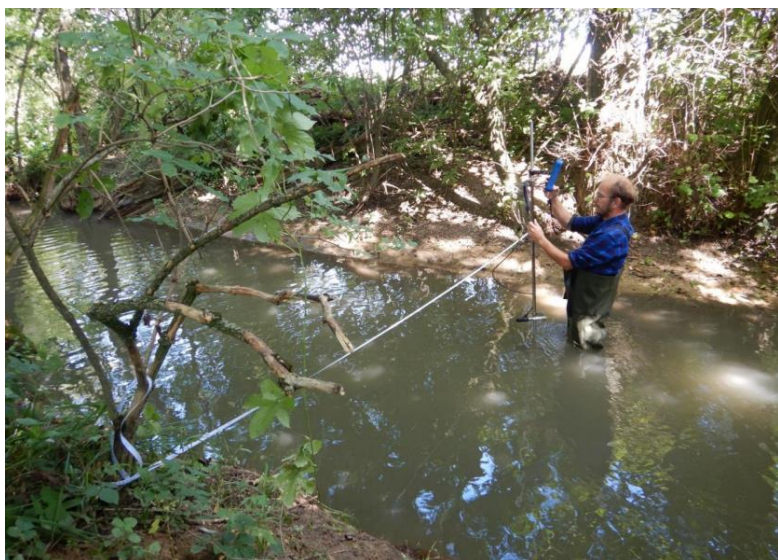
Discharge measurements at the surface stream Horná Blava below the Dechtické pramenisko linear spring. Photo: Peter Malík
