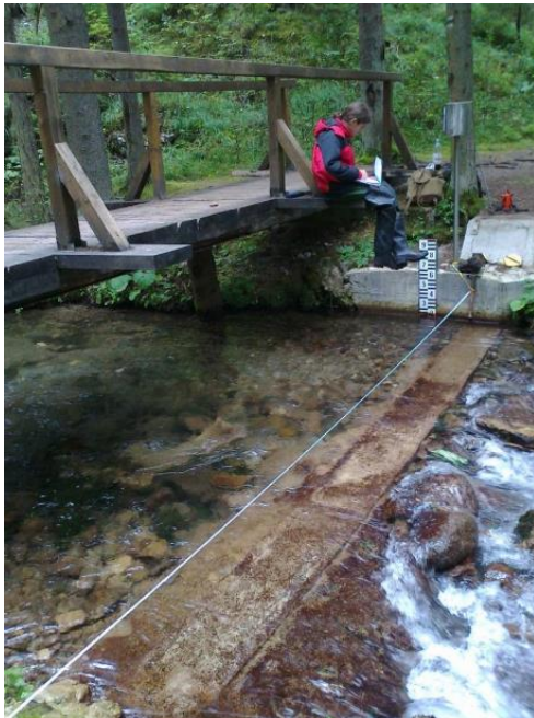
Gauging object for discharge monitoring at the Vyvieranie spring, photo: František Bottlík
