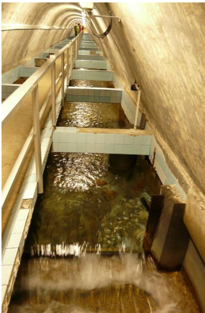
The flow measurement device (Poncelet's weir) at the end of the Lazce spring collection gallery. Photo: Peter Bajtoš.
