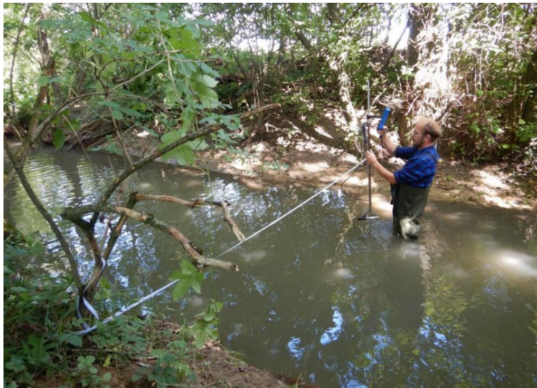
Discharge measurements at the surface stream Horná Blava below the Dechtické pramenisko linear spring. Photo: Peter Malík
