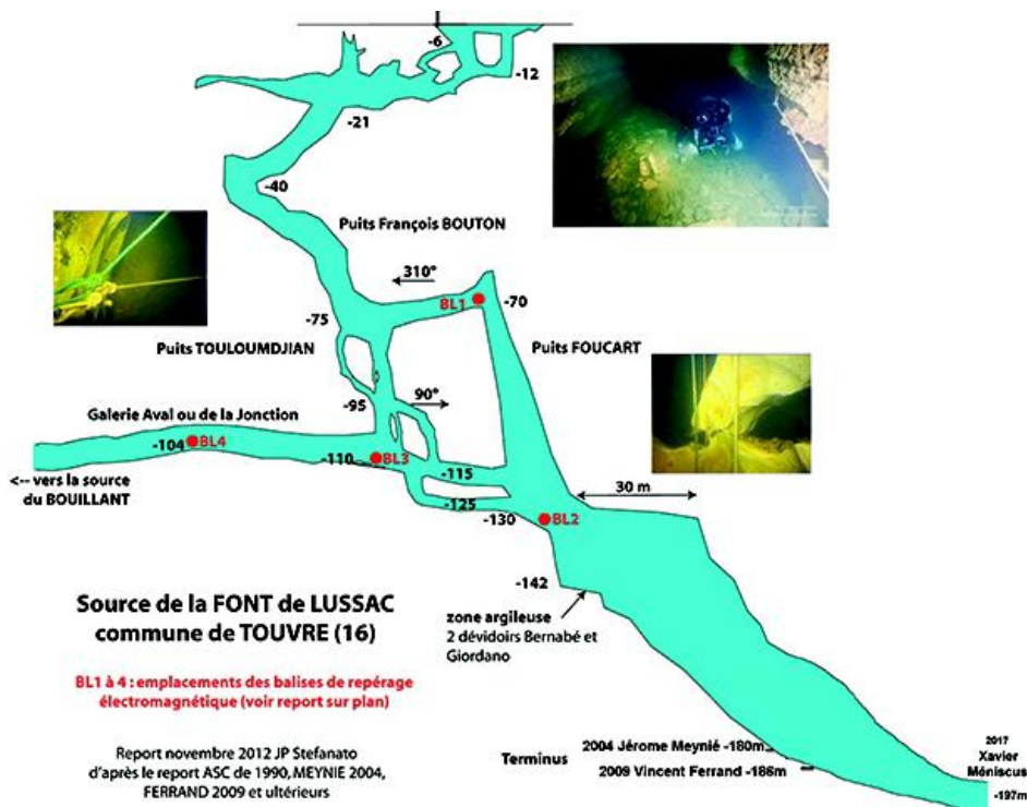
Cross-section of the Font de Lussac, one of the Touvre springs ( https://subaqua.ffessm.fr/article/les-sources-de-la-touvre/ )
